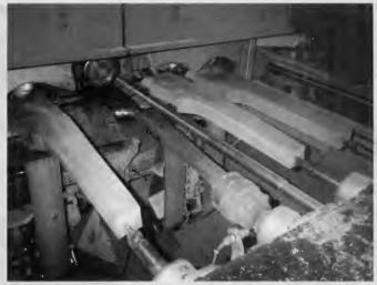
(above) The receiver is milled from solid steel bar stock on CNC machinery. (above, right) Stock blanks are roughed out on automatic equipment. (far right) Highly skilled artisans hand-fit the barreled actions to the stock using smoke from a kerosene lamp that is re-applied until the fit is perfect. (right) Vektor's engraver works on a floorplate for a custom rifle. High quality engraving is available on special order.
